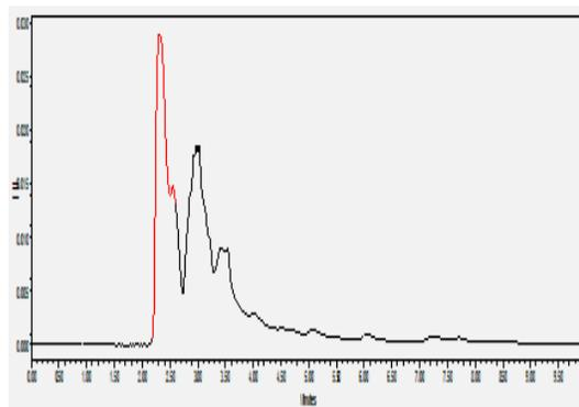
**Figure 3: Chromatogram of blank unspiked rat plasma sample manifests the selectivity of the method which displays the lack of interfering peaks at the retention time of the assayed drugs and the internal standard in the chromatogram.**
