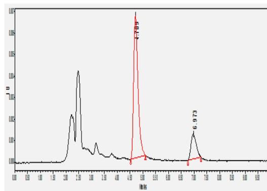
**Figure 2: Chromatogram of analyte Cyproheptadine HCl and internal standard Oxcarbazepine spiked in human plasma showing the development of HPLC method after application of liquid liquid extraction method. The peak at retention time of 6.8 represents analyte Cyproheptadine HCl (CPH), the peak at retention time of 4.7 min represents internal standard Oxcarbazepine (OXZ) and peak at retention time of 2 min is for plasma interference.**
