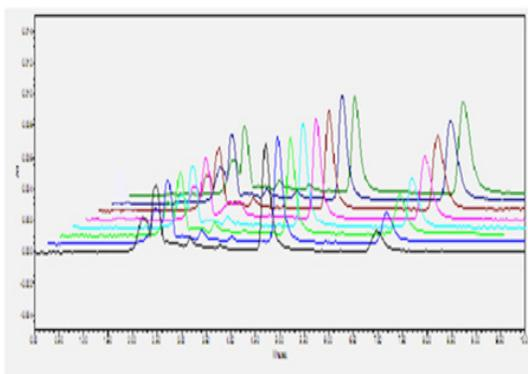
**Figure 1: Overlain Chromatogram of Analyte Cyproheptadine HCl (CPH) and Oxcarbazepine (OXZ) used as Internal standard in developed HPLC method (800ng/ml - 100ng/ml is the concentration range of analyte whereas the concentration of Internal standard used is 100 ng/ml). In the chromatogram the peak at retention time of 4.7 min denotes internal standard and peak at retention time of 6.8 min denotes analyte.**
