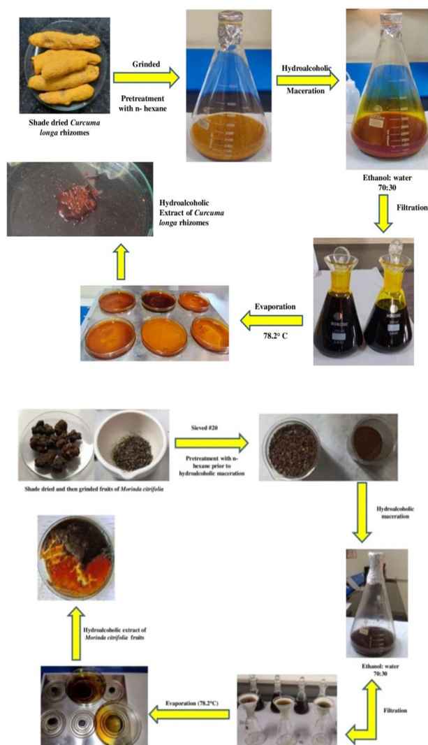
Figure 2: Hydro-alcoholic maceration of Curcuma longa rhizomes (2A) and Morinda citrifolia fruits (2B).
