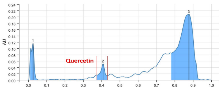
Figure 5A: HPTLC Chromatogram of methanolic extract of Linum usitatissimum L. (Flax) Seeds.
