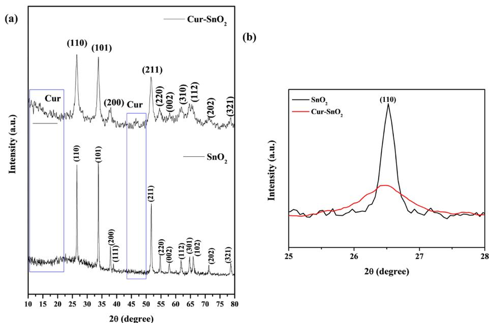
**Figure 1:** (a) XRD pattern of SnO<sub>2</sub> and Curcumin-SnO<sub>2</sub> NPs and (b) Enlarged patterns of SnO<sub>2</sub> and Curcumin-SnO<sub>2</sub> NPs at 25 to 28°.
