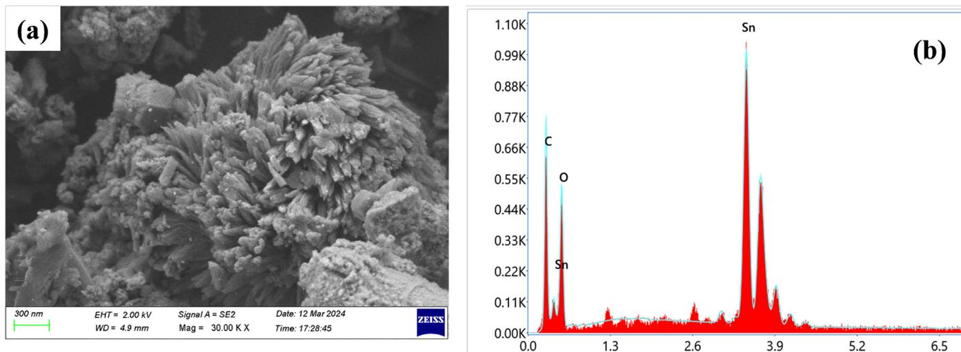
**Figure 2:** (a) FE-SEM and (b) EDAX spectra of Curcumin-SnO<sub>2</sub> NPs.
