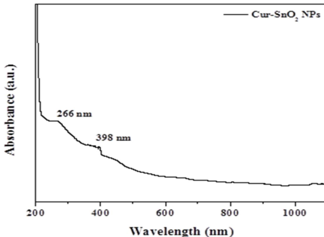
**Figure 3:** UV-vis absorbance spectrum of Curcumin-SnO<sub>2</sub> NPs.
